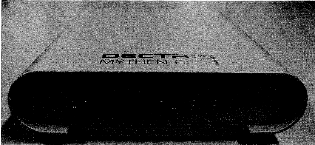
Figure 3: Front panel of the detector control system 1.
